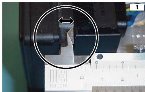
**ES WIRD EMPFOHLEN, EINE SCHABLONE ANZUFERTIGEN, UM DAS KORREKTE EINSETZEN DES KABELSTECKERS ZU PRÜFEN.**
