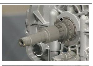
• Place the camshaft with the reference pin of the gear pointing downwards.
