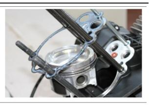
• Place a commercially available appropriate ring clamp on the piston.
