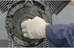
• Unscrew the screws securing the pressure plate flywheel to the crankshaft and then remove it.
