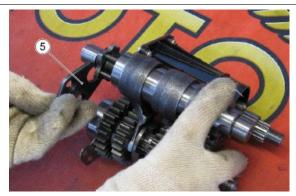
• Release the main shaft (6) and the transmission shaft (7) from the forks
