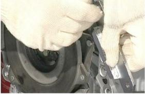
• Tighten the screws following a crisscross pattern with a torque wrench set to the prescribed torque. It is advisable to change the fixing screws securing flywheel to crankshaft.
