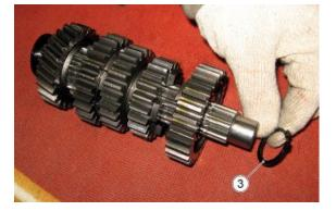
Remove the spacer (4) • Remove the gear of the 6th gear (5) ٠ 5 Remove the bushing (6) ٠ 6 Remove the spacer (7) •
