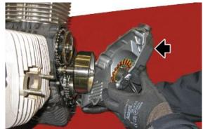
Remove the rotor fixing screw • Insert in the rotor hole the specific ٠ spacer Place and tighten the tool (1) on the ro-٠ tor.
