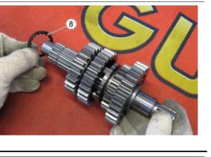
• Remove the gear of the 4th gear (9)
