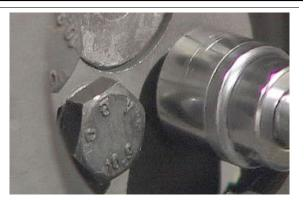
• Insert the clutch engagement/disengagement cap with its retainer ring.
