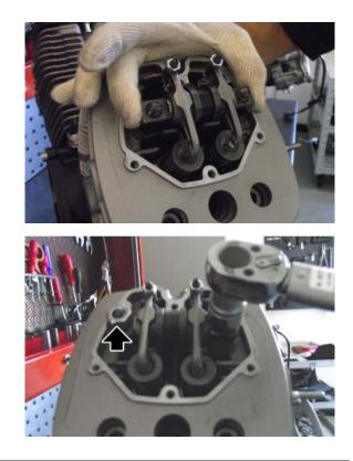
• Tighten the nuts to the prescribed torque following a crisscross pattern.
