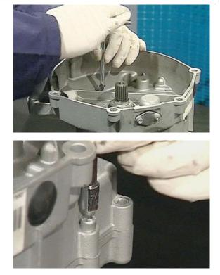
Detach and remove the clutch bell together with the clutch shaft tapping lightly around clutch bell edge.
