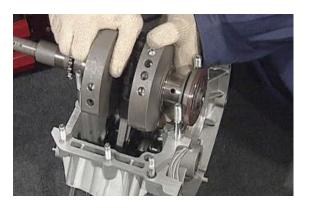
Fit the half-bearings (lubricate them first) into the lower crankcase; apply the specified liquid gasket to the crankcase mating faces
