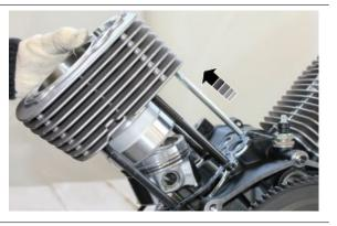
• Remove the gasket from the stud bolts
