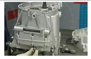
• Unscrew the gearbox cover bolts and remove the cover tapping it with a mallet.
