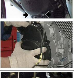
• Unscrew the screws fixing the stator to the timing system cover and slide off the stator.
