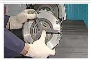
• Fit the assembly on the pressure plate flywheel and tighten the screws to the prescribed torque.
