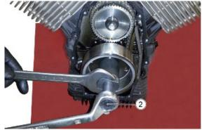
Operating on the alternator cover, proceed with the removal of the stator wiring lock plate
