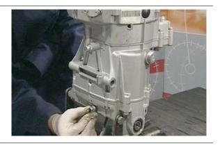
Insert the clutch control rod into the shaft with the larger diameter facing the control lever.
