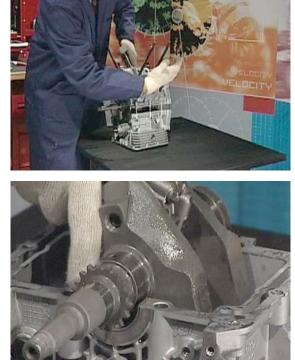
Unscrew the oil pressure sensor from the upper crankcase and remove the retaining bushing of the camshaft; remove the shaft and the tappets, noting their positions.
