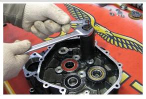
Remove the drive shaft secondary oil gaiter
