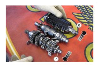
Remove the upper fork (6) from the desmodromic shaft by sliding the guide towards the grooves of the guide itself
