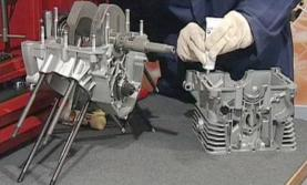
• Join the two crankcase halves and tap lightly with a mallet to ensure that the two mating faces adhere together firmly; tighten the four central stud bolts and the external nuts following a crisscross pattern.
