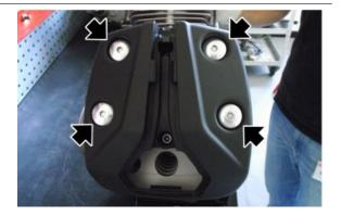
• Loosen the central fastening screws
