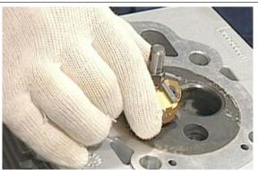
Insert the T handle into the cutter and turn clockwise while pressing lightly achieving an even valve contact surface.
