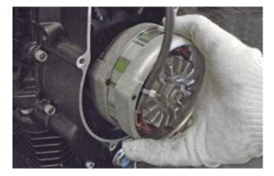
• Unscrew the nut fixing the rotor to the crankshaft, slide off the rotor, remove the key and collect the washer.
