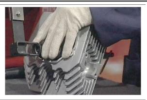
• Slide off the upper cap, the spring and finally the valve.
