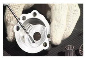
External rotor seat thickness 15.030 -15.070 mm (0.5917 - 0.5933 in).
