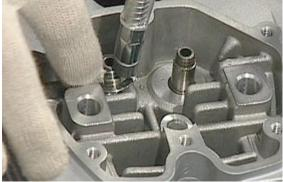
Valve guides need to be knocked out tapping from the inside with punch and mallet; heat the head up to approximately 50-60 °C to aid removal.
