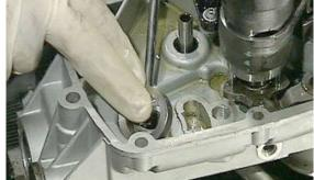
After unscrewing the retaining plate fixing screws, remove the complete set of gears, shafts and forks.
