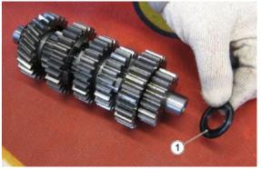
• Remove the gear of the 2nd gear (2)
