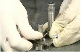
• Remove the counter nut and the fixing nut of the eccentric screw
