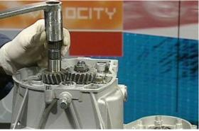
• Unscrew the transmission gear retaining nut and slide off the thrust washer.
