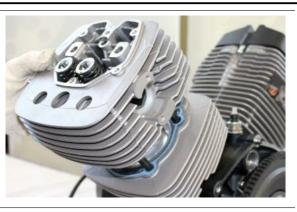
• Remove the cylinder head gasket
