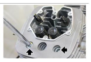
Remove the complete head from the cylinder
