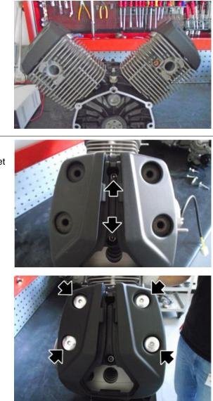
• Tighten the screws following a crisscross pattern with a torque wrench set to the prescribed torque.
