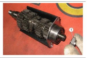
• Remove the bearing (2) using a generic bearing extractor
