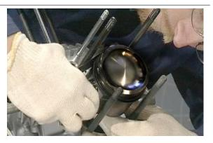
When finished, remove the tool and insert the second snap ring that closes the piston pin seat, after protecting the cylinder seat.
