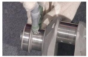
The maximum parallelism deviation of the two crankshaft axes (connecting rod pin and main journals on flywheel side and timing system side) should not exceed 0.02 mm (0.0009 in) at 40 mm (1.5748 in) distance.
