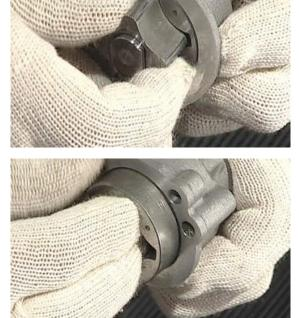
• Slide off the bearings and their inner housing from pump body.
