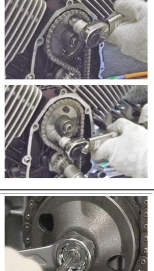
• Tighten the oil pump nut while holding the oil pump shaft steady.
