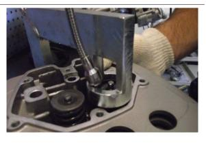
• Unscrew the tool and remove it from the head.
