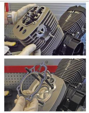
• Fit the rocker lower spacers, the rocker control rods, the rockers and the upper spacers with their nuts.
