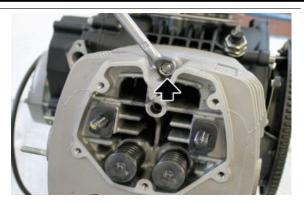
• Remove the internal screws fixing the head to the cylinder
