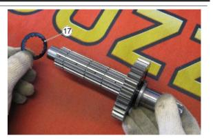
• Remove the gear of the 2nd gear (18)
