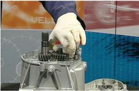
• Remove the gear and the clutch shaft.
