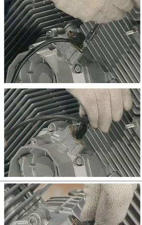
Position the engine speed sensor on the timing system cover and tighten the two fastening screws to the prescribed torque.
