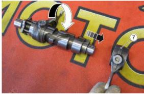
Remove the lower fork (8) from the desmodromic shaft by turning and sliding the guide towards the grooves of the guide itself
