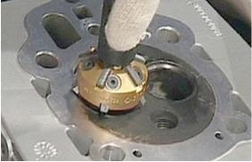
• Repeat the procedure using the suitable cutter to achieve the correct valve seat sealing surface.
