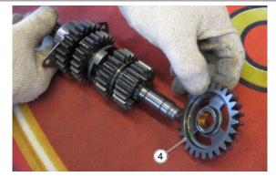
• Remove the gear of the 5th gear (5)
