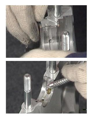
Insert the seal ring (after lubricating it) on the crankshaft and the assembly onto the engine crankcase making sure that the connecting rods locate correctly into their seats.
