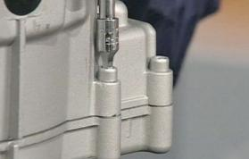
• Tighten the clutch shaft nut using the suitable tool and squash.
