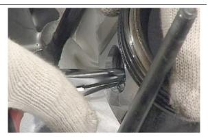
• Slide off the pin using the specified tool (turn the tool screw) and remove the piston.
