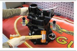
• To remove the bearings fitted in the gearbox crankcases, the safety washer must be removed first
