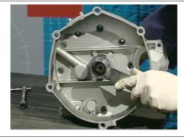
• Slide off the clutch shaft and remove the seal ring.
