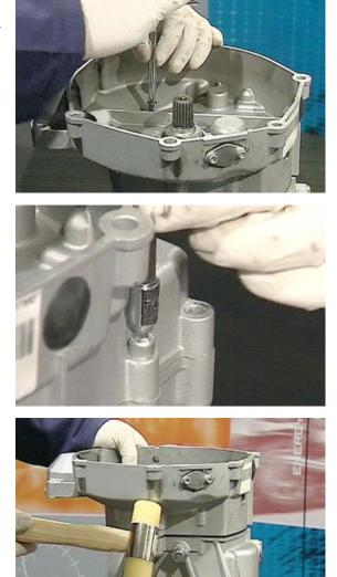
Slacken the lock nut and unscrew the pre-selector positioning eccentric screw.
