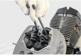
Remove the outer nuts that fix the head to the cylinder and collect the washer
