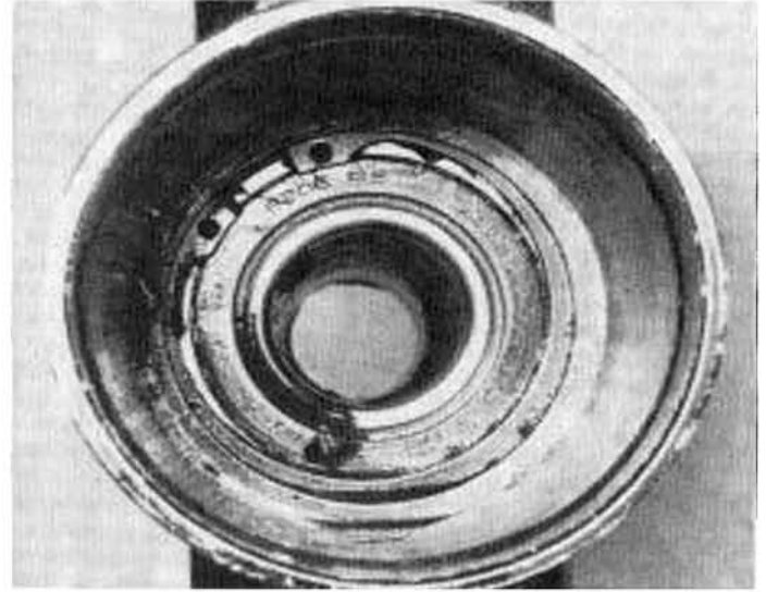
9.3 Shaft bearing is retained by a circlip
