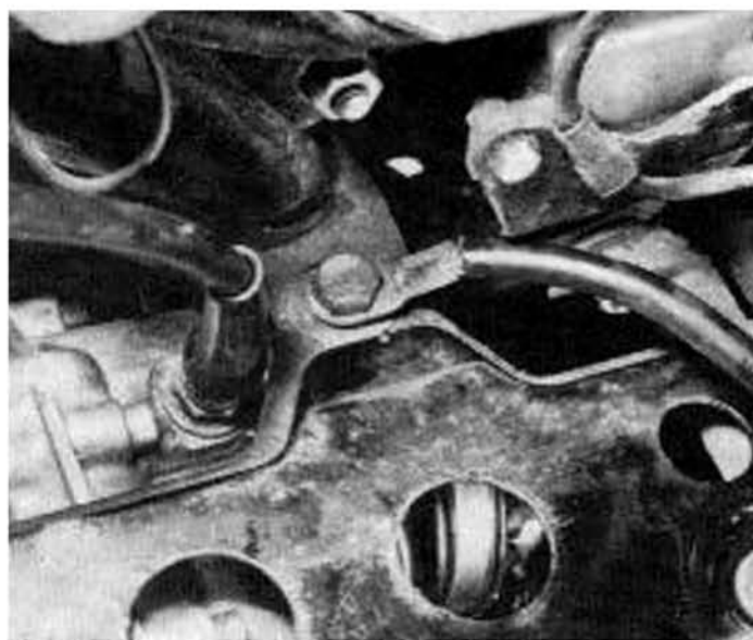
4.16b ... the bolt which holds the battery earth lead
