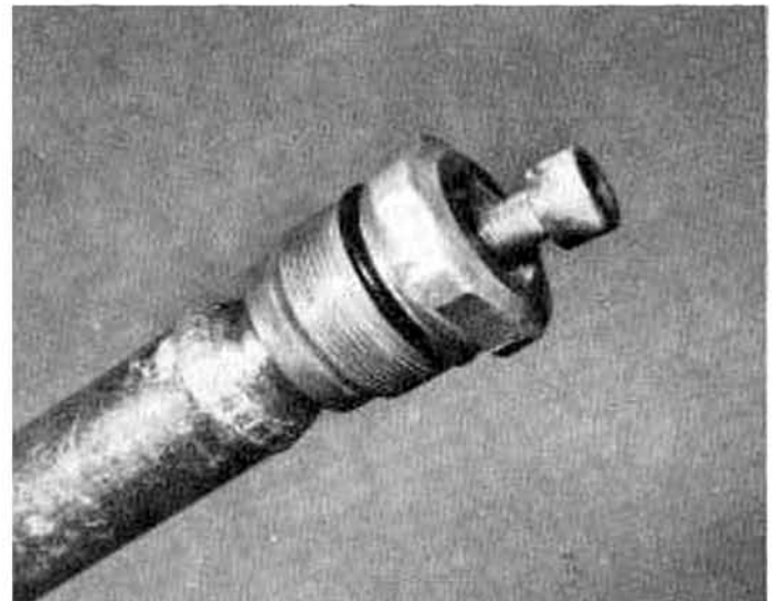
3.2b ... retained by a socket screw
