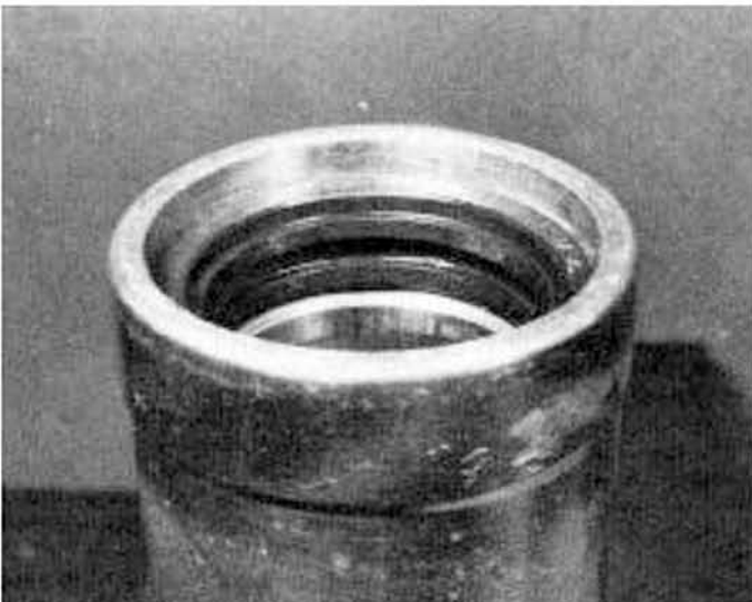
4.4 Double oil seals can be prised out
