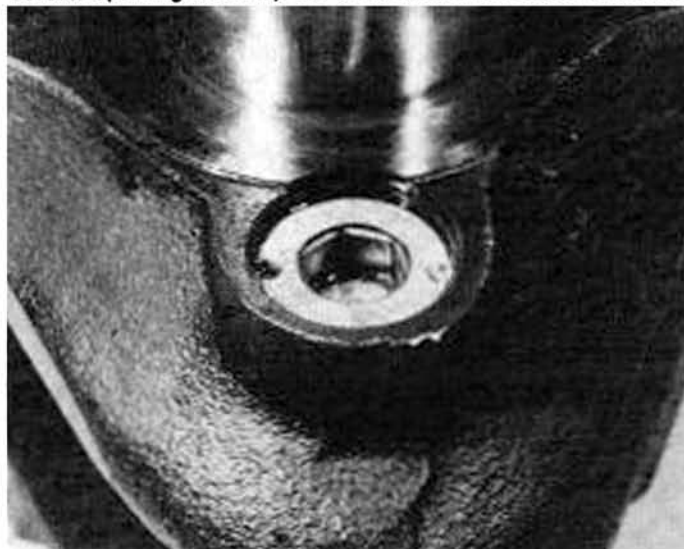
25.1 Crankshaft plug must be absolutely tight
