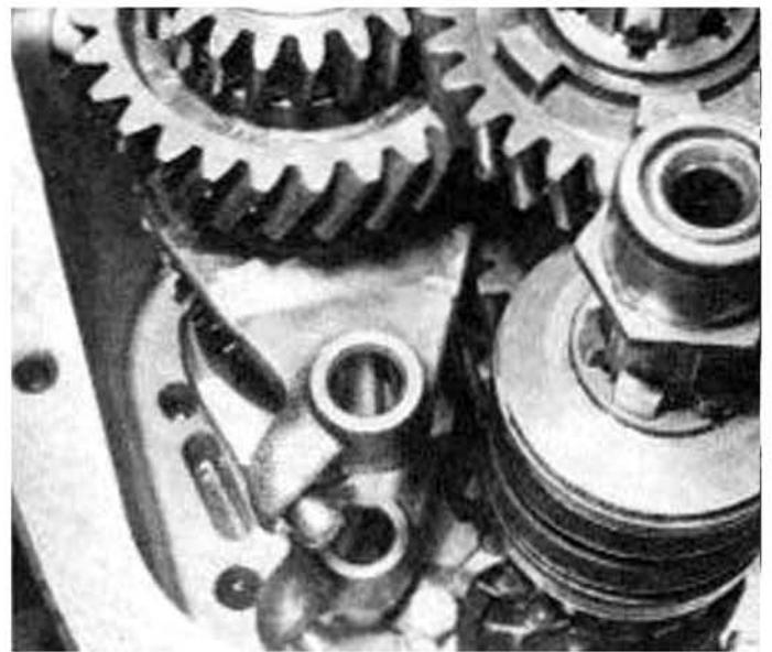
7.5a Fit the two mainshaft selector forks and ...
