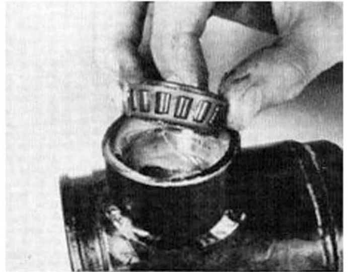
8.14a Grease the tapered bearing thoroughly
