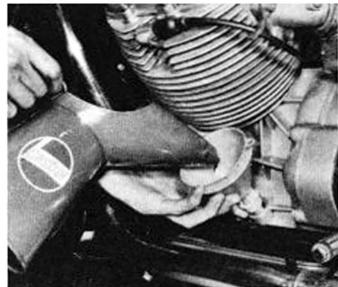
Check and if necessary replenish engine oil
