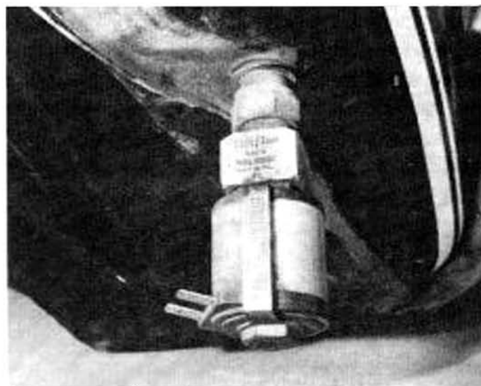
2.1 'Electrovalve' ignition operated petrol tap
