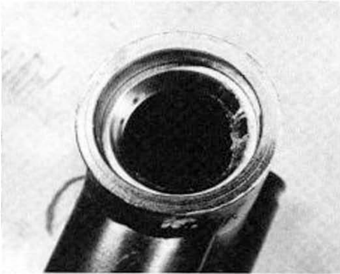
8.13 Check the outer races for indentation and scoring
