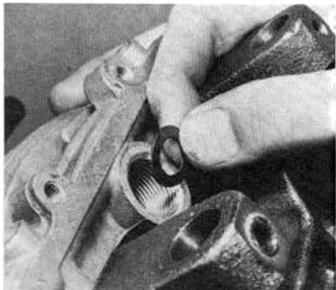
27.8d Small washer fits on short upper stud below ...
