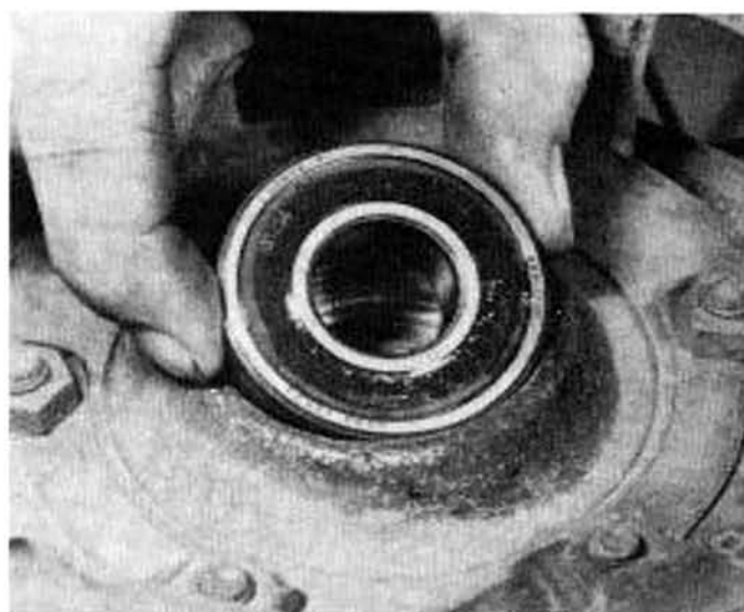
10.2b Bearings may be drifted out
