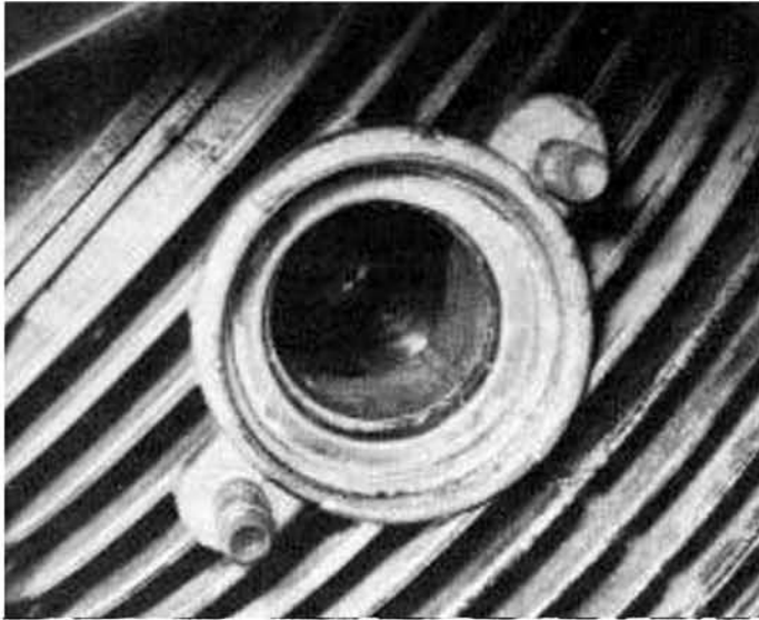
33.4a Insert a new ring gasket into each port
