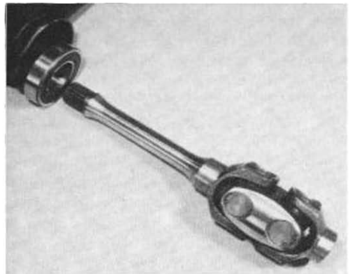
9.1a One piece final drive shaft - V-1000 models
