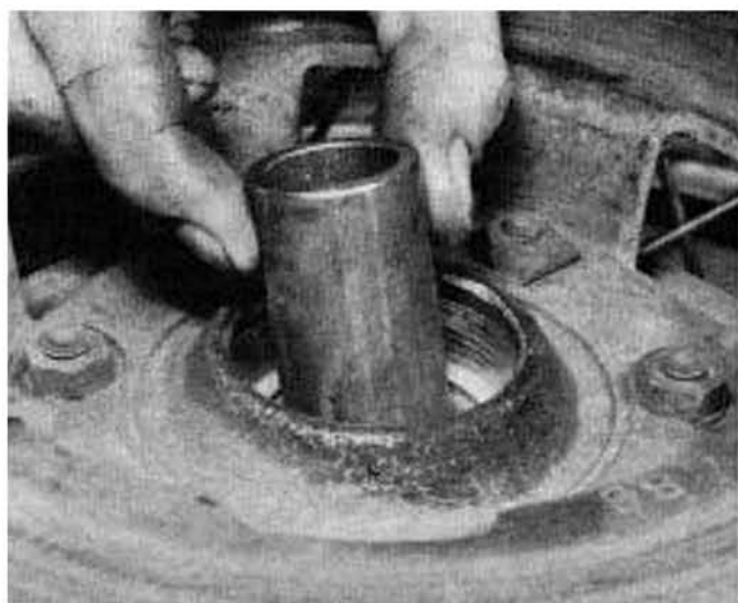
10.2c Note the bearing spacer; it must not be omitted
