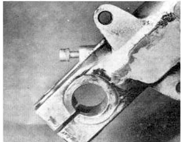
3.1 Lubricate drain plug in the base of each leg
