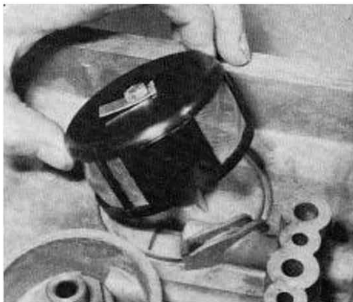
Detach and clean oil filter screen
