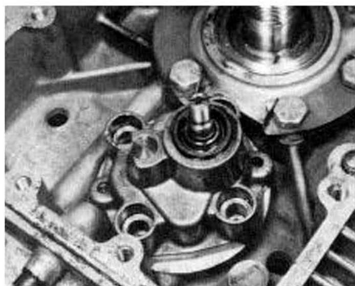
10.1 Oil pump secured by four screws, located on two dowels
