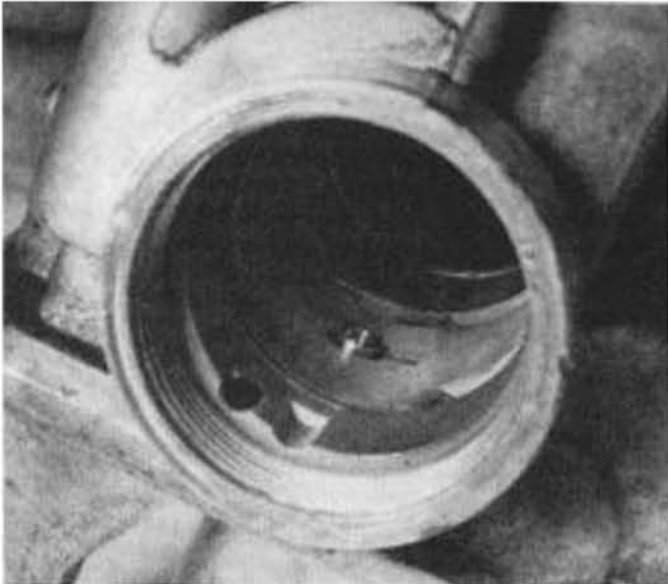
4.3e Push down the main nozzle and ...
