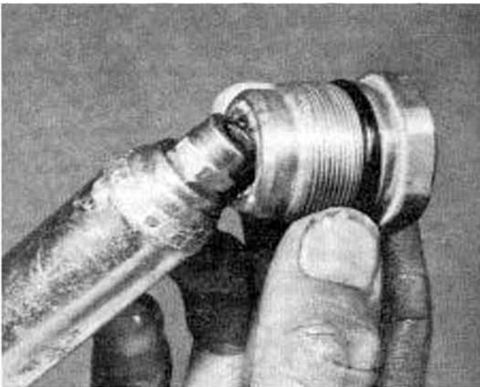
3.2a Damper unit seats in fork top bolt and is ...
