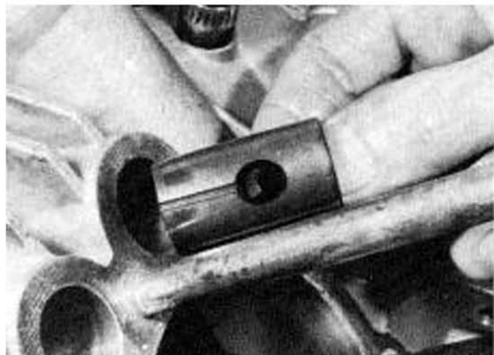
27.2 Lubricate and fit cam follower in original positions
