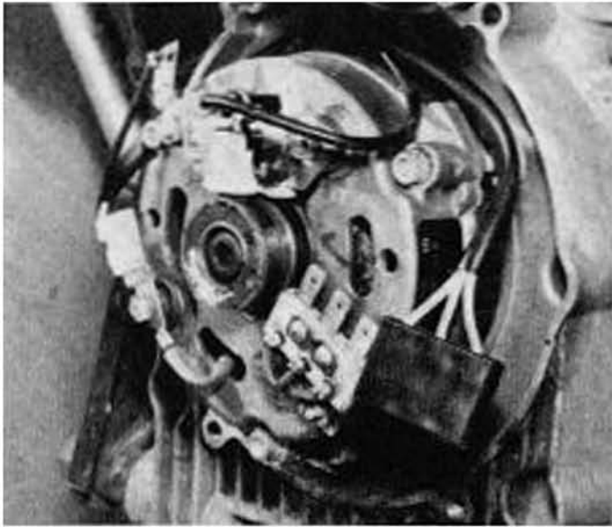
5.4a Note alternator wiring before removal
