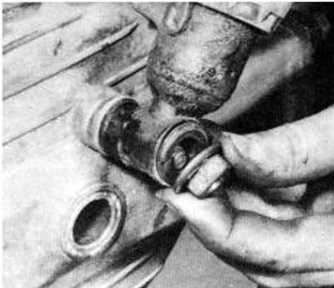
8.7b ... by a nut on a stud. Note split rubber bushes
