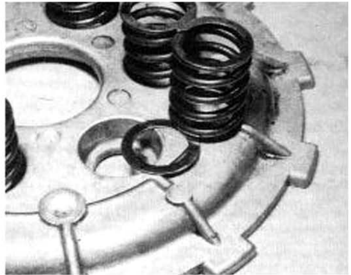
11.5b Note the shims between plate and springs
