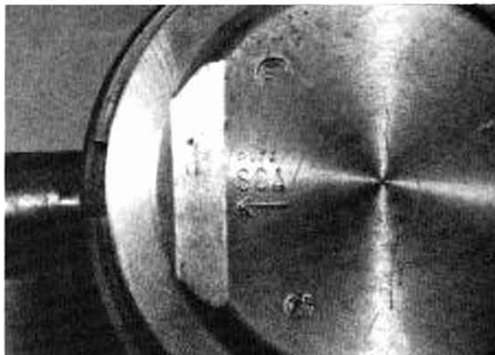
27.4a Arrow on piston must face forwards
