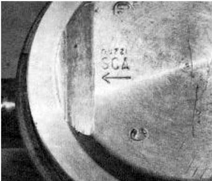
19.2 Mark 'C' on piston indicates cylinder/piston classification
