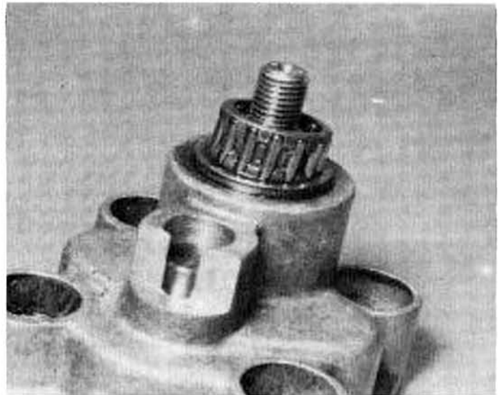
10.2c The double row roller bearing can be pushed out
