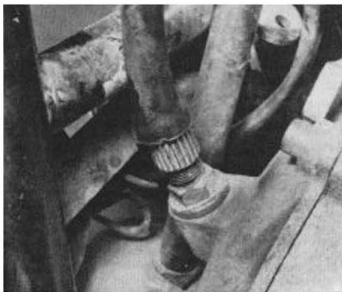
4.12a Unscrew tachometer cable followed by ...
