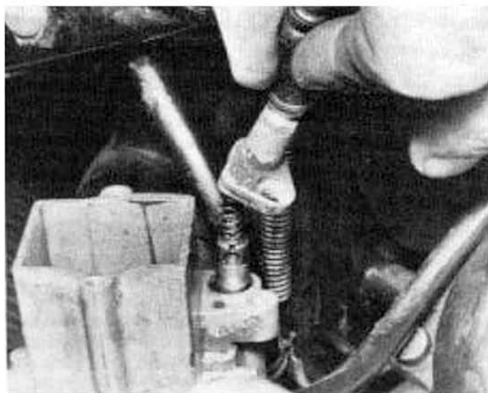
3.2d Choke plunger housing held by a single screw
