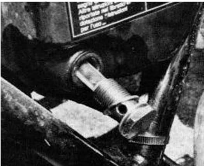
16.2 Lower pipe banjo bolt incorporates filter screen
