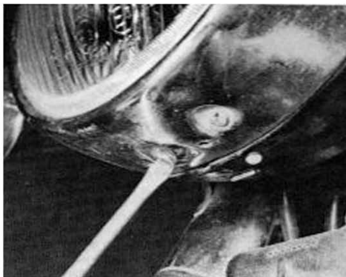
9.1 Headlamp rim held by single screw - except 750 models
