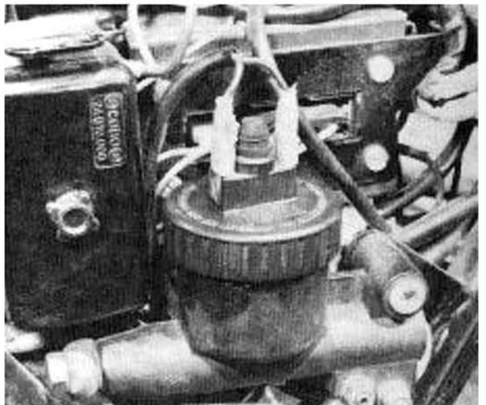
15.4a Fluid level switch on V-1000 models is ...
