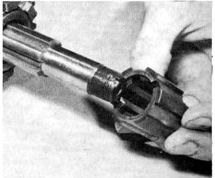
4.3f ... internally and externally splined sleeve
