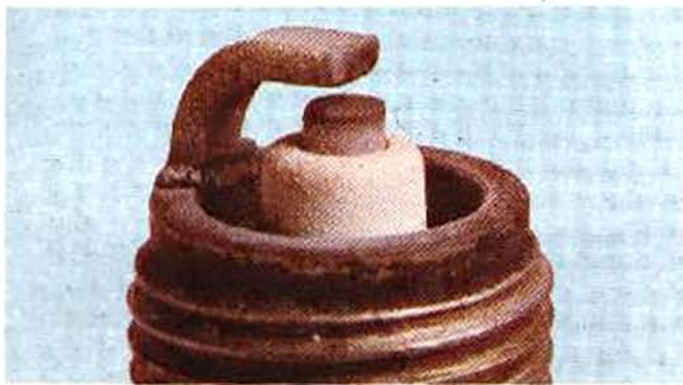
Spark plug conditions: A brown, tan or gray firing end is indicative of correct engine running conditions and the selection of the appropriate heat rating plug
