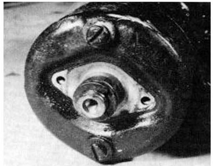
11.2b ... prise off the circlip and washer
