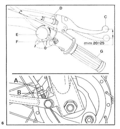
loosening counternut «B» (Pict.6). The idle movement must be 20-25 mm. The lever «C» actuates the stoplight cutout (D) and the tail light bulb «D» Pict. 10 lights on;
