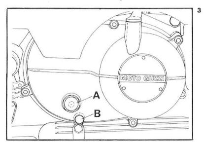
the crankcase very well before adding fresh oil. «A» filling cap; «B» draining plug.
