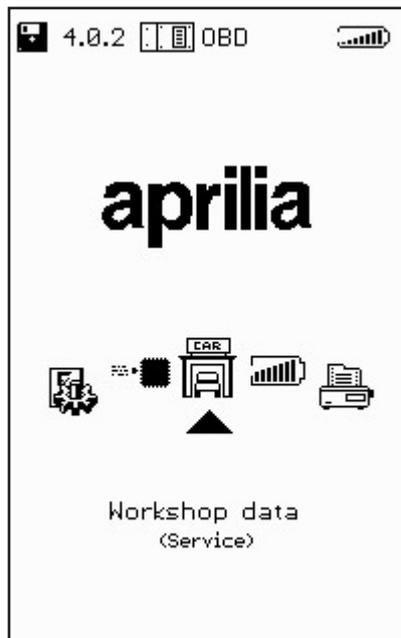
This function is used to enter the name of the workshop which will appear in the main menu when the AXONE2000 APRILIA is switched on.
