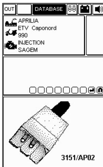
Connect the adapter cable to the ECU auto-diagnostic socket as shown in the figure using the suggested connection cable.
