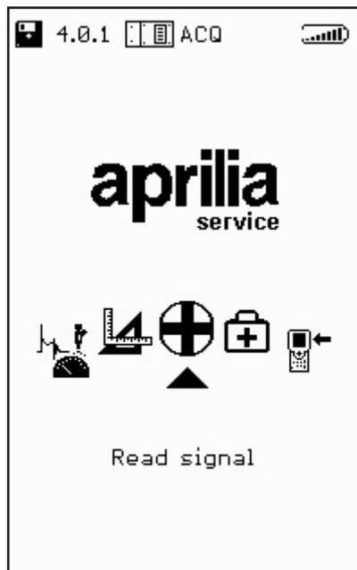
Use the left/right scroll arrows to scroll the icons of the tool/function to be selected and then press ENTER to confirm.
