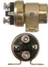
131253 Solenoid Replacing: 19024762 12 V., 60 Amp., Intermittent load 500 Amp., Seconds 5, Coil bolt M8
