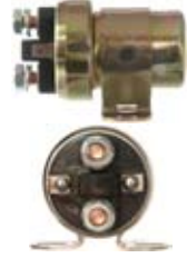
131254 Solenoid Replacing: 19024763 24 V., 50 Amp., Intermittent load 500 Amp., Seconds 5, Coil bolt M8
