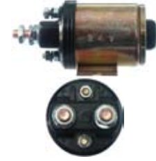
133697 Solenoid Replacing: CEZ113, 098932 24 V., 100 Amp., Intermittent load 500 Amp., Seconds 5, Coil bolt M8
