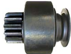
136502# Drive Replacing: 1360-001-00X0 Servicing: 0300-552-0011, 28100-1400 O.D. 46.50, I.D. 19.10, L. 91.45, Teeth 13, Splines 18
