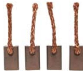
140357 Brush Set Replacing: TAJ400 12 V., L. 18.99, Th. 6.88, H. 11.91
