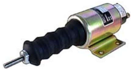
090168 Shut Down Solenoid 12V Servicing: UNIVERSAL. 12 V., 0.63 Amp., 6.00, Stop solenoid35 Newton178 Newton75 Newton Syncro start / Woodward.
