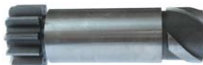
131714 Drive Replacing: 18.100.021 Servicing: 11.130.158 O.D. 41.00, I.D. 14.60, L. 120.00, Teeth 11, Splines 1 3
