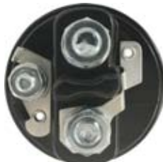
138003 Solenoid Cap Servicing: 0331303133, 0331303142, 0331303159, 0331303659, 2339303201, 2339303206 O.D. 54.25, Terminals 3
