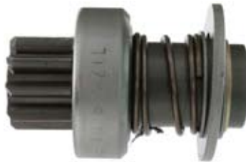
130730 Drive Replacing: 17061-8, 17061-2 Servicing: MTA12-13, MTA12-20, MTA12-42, MTA12-5, MTA12-7, MTV12-5, MTV12-7 O.D. 25.25, I.D. 11.55, L. 62.15, Teeth 9, Splines 12, Rotation ACR
