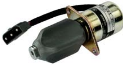
090226 Shut Down Solenoid 24V 24 V., 0.5 Amp., 6.00, Stop solenoid7 Newton182 Newton111 Newton Syncro start / Woodward. Red=Common. White=Pull. Yellow=Hold.
