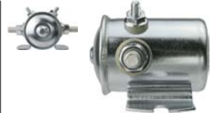
235647 Solenoid 36 V., 60 Amp., Intermittent load 150 Amp., Seconds 5 Insulated return.
