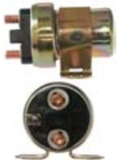
130492 Solenoid Replacing: 19024765 24 V., 50 Amp., Intermittent load 500 Amp., Seconds 5, Coil bolt M8
