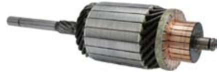
230855 Armature Replacing: 16.361.103 Servicing: 11.130.665, 11.130.694, 11.130.709, 11.130.736, 11.130.795, 11.130.811, 11.130.889, 11.130.895, 11.130.995, AZJ3217 12 V., 2.7 kW., Shaft L. 309.96, Splines 10, Rotation CR
