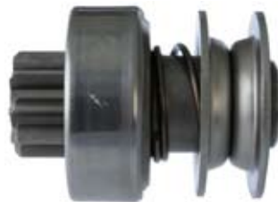
130434 Drive Replacing: 079692 Servicing: 532001B, 532017A O.D. 25.30, I.D. 12.00, L. 61.70, Teeth 9, Splines1 9, Rotation CR
