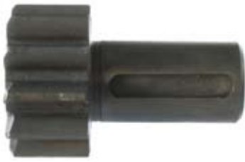
130418 Drive Replacing: 15.100.152 O.D. 41.00, I.D. 10.15, L. 61.00, Shaft L. 39.65, Teeth 11
