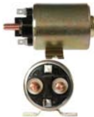
131371 Solenoid Replacing: 333006006 Servicing: 333006006 24 V., 80 Amp., Intermittent load 500 Amp., Seconds 5, Coil bolt M8 Silver contact. Insulated return.
