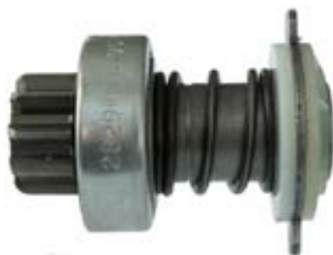
130740 Drive Replacing: 16.900.038 O.D. 25.30, I.D. 11.50, L. 65.00, Teeth 9, Splines 1 2, Rotation ACR
