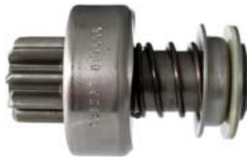
131267 Drive Replacing: 16.903.130 O.D. 34.80, I.D. 14.00, L. 91.00, Teeth 9, Splines 1 10, Rotation CR
