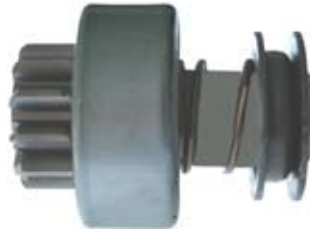
132515 Drive Replacing: 0-23500-0523, 0-23500-0520 Servicing: 0-23000-0250, 0-23000-0250, 0-23000-0272, 0-23000-0283, 0-23000-0370 O.D. 40.40, I.D. 13.85, L. 81.00, Teeth 11, Splines 12, Rotation CR
