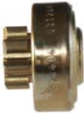
234404 Drive Servicing: 228000-6240 O.D. 27.65, I.D. 12.00, L. 33.65, Teeth 8, Splines 6 Bronze.
