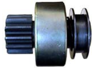
132519 Drive Replacing: 1-23500-0170 Servicing: 0-23000-3150, 0-23000-3152, 0-23000-3180, 0-23000-3270, 0-23000-3280, 0-23000-3285, 0-23000-3291, 0-23000-3301 O.D. 46.50, I.D. 19.32, L. 96.50, Teeth 12, Splines 15, Rotation CR
