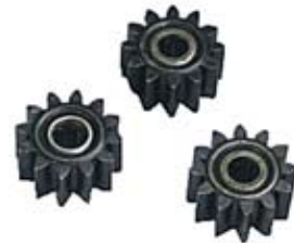
139572 Gear Wheel Kit O.D. 18.00, I.D. 5.00, H. 9.50, Teeth 12
