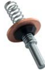
139853 Moving Contact Servicing: 2250-27002, 2250-27003 L. 26.00, Th. 2.25, Shaft measurement 33.40 Silver plated.
