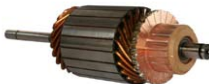
136106 Armature Servicing: 0001362600, 0001362601, 0001362605 9 V., 2.3 kW., Shaft L. 285.00, Splines 10, Rotation CR 12V: Cargo 136105.
