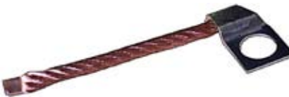
134921 Terminal Lead Servicing: M10. I.D. 10.35, Lead L. 68.20
