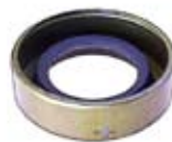
132382 Oil Seal Replacing: 1918047 Servicing: 40MT, 42MT, 50MT., 10461041, 10461045, 10461046, 10461047, 10461048, 10461059, 10461060, 10461061, 10478800, 10478801 O.D. 34.90, I.D. 19.50, H. 9.50
