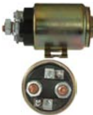
131373 Solenoid Replacing: 333009004 Servicing: 333009004 12 V., 150 Amp., Intermittent load 800 Amp., Seconds 5, Coil bolt M8 Silver contact. Insulated return.
