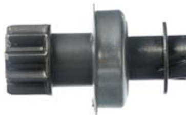
234970 Drive Replacing: 028300-6010 Servicing: 128000-1870, 128000-4870, 128000-7480, 228000-0120, 228000-2640, 228000-7990, 228000-9261, 280000-2640, 280000-7190 O.D. 28.85, I.D. 13.00, L. 75.00, Teeth 9, Splines 5, Rotation ACR
