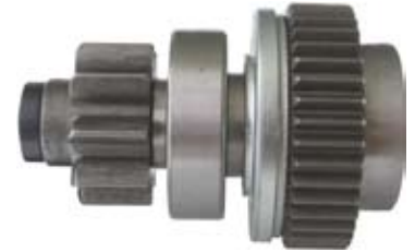
235101 Drive Servicing: 228000-7220 O.D. 35.45, L. 83.00, Teeth 9, Splines 10, Rotation CR
