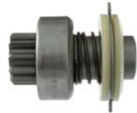
130738 Drive Replacing: 17061-10 Servicing: MTD12-14, MTD12-19, MTD12-9 O.D. 29.15, I.D. 14.00, L. 68.00, Teeth 11, Splines 6, Rotation CR
