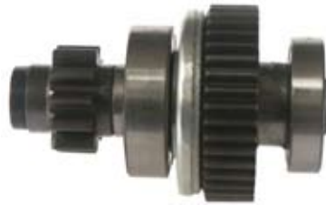
234905 Drive Servicing: 128000-8110, 128000-8111 O.D. 29.75, L. 87.00, Teeth 11, Splines 10, Rotation CR
