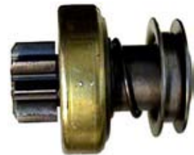
133291 Drive Replacing: 0-23500-0422, 0-23500-0421, 0-23500-0420 Servicing: 0-23000-0091, 0-23000-0091, 0-23000-0172, 0-23000-0172, 0-23000-0173, 0-23000-0260, 0-23000-0260, 0-23000-0262 O.D. 32.50, I.D. 13.10, L. 71.00, Teeth 9, Splines 12, Rotation CR
