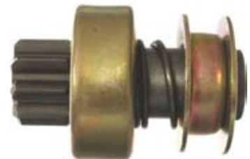
132764 Drive Replacing: 16.900.089 Servicing: 11.130.029, 11.130.102, 11.130.162, 11.130.166, 11.130.209, 11.130.217, 11.130.218, 11.130.219, 11.130.234, 11.130.293 O.D. 25.15, I.D. 11.60, L. 65.00, Teeth 9, Splines 1 12, Rotation CR
