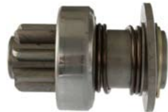
130920 Drive Replacing: 9586-1, 9328 Servicing: MTA12-1, MTC252-2, MTC252-6, MTC252-7, MTC402-15, MTC402-2 O.D. 26.95, I.D. 12.00, L. 60.65, Teeth 8, Splines 6, Rotation ACR
