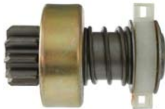
130733# Drive Replacing: 17061-16 Servicing: MOA12-10 O.D. 26.70, I.D. 12.00, L. 67.15, Teeth 10, Splines 12, Rotation CR
