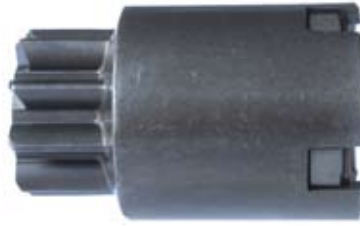
130449 Drive Replacing: 14898-1 Servicing: MTJ12-1, MTU12-1 O.D. 29.10, I.D. 16.00, L. 58.00, Teeth 9, Splines 4, Rotation ACR
