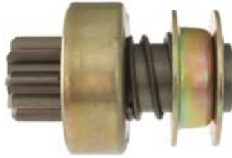
130754# Drive Replacing: 18.900.383 Servicing: 10.130.100 O.D. 25.25, I.D. 11.50, L. 65.00, Teeth 9, Splines 1 12, Rotation CR
