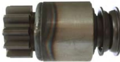
132516 Drive Replacing: 1-21500-1530, 1-12500-1530 Servicing: 0-21000-3390, 0-21000-3391, 0-21000-4890, 0-21000-5080, 0-21000-5210 O.D. 56.85, I.D. 18.00/20.00, L. 115.00, Teeth 11, Splines 15
