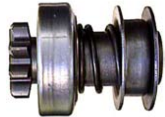
132624# Drive Replacing: 18.900.297 Servicing: 10.130.072 O.D. 29.00, I.D. 11.50, L. 58.00, Teeth 9, Splines 1 12, Rotation ACR
