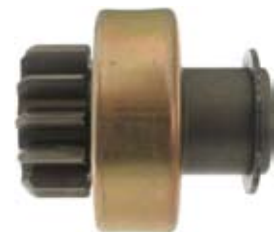
237880 Drive Servicing: 428000-1620 O.D. 32.50, L. 50.50, Teeth 12, Splines 10
