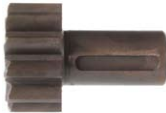
131167 Drive Replacing: 15.100.154 O.D. 42.00, I.D. 10.15, L. 61.00, Shaft L. 40.00, Teeth 11
