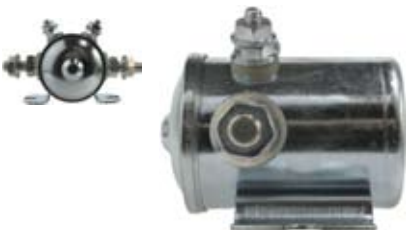
235443 Solenoid 24 V., 100 Amp., Intermittent load 200 Amp., Seconds 5 Silver contact. Insulated return.
