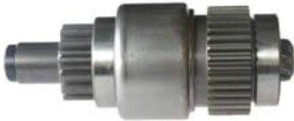
234683 Drive Replacing: 028300-6731, 028300-6730, 028300-3731 Servicing: 228000-4680, 228000-6470, 228000-6471 O.D. 39.20, L. 146.70, Teeth 13, Splines 10
