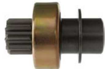
130463 Drive Replacing: 095381, 093321, 092448, 092181, 079011, 078861, 077776 Servicing: D8E107, D8E115, D8E117, D8E129, D8E133, D8E134, D8E137, D8E139, D8E147, D8E151, D8E54, D9E11, D9E18, D9E19, D9E27 O.D. 25.30, I.D. 12.00, L. 66.40, Teeth 9, Splines1 12, Rotation CR
