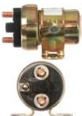
131080 Solenoid Replacing: 19024764 12 V., 50 Amp., Intermittent load 500 Amp., Seconds 5, Coil bolt M8
