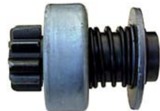
131064 Drive Replacing: 17061-25 Servicing: MTA12-40 O.D. 27.95, I.D. 11.55, L. 61.90, Teeth 10, Splines 12, Rotation ACR
