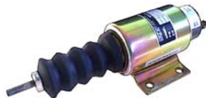
090113 Shut Down Solenoid 24V Servicing: EXTERNAL. 24 V., 0.3 Amp., 6.00, Stop solenoid35 Newton178 Newton75 Newton Syncro start / Woodward.
