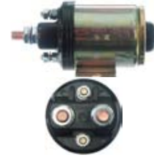
133695 Solenoid Replacing: CEY113, 099845 12 V., 100 Amp., Intermittent load 500 Amp., Seconds 5, Coil bolt M8
