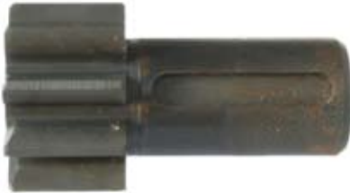
130419 Drive Replacing: 15.100.092 O.D. 35.00, I.D. 10.60, L. 61.20, Shaft L. 40.10, Teeth 9
