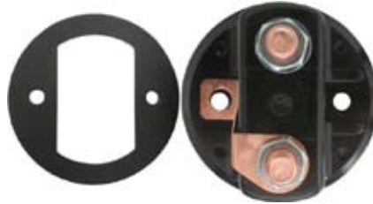
134401 Solenoid Cap Servicing: 073302, 182438, CED501, CED539 O.D. 60.60, Terminals 3 w/ gasket.
