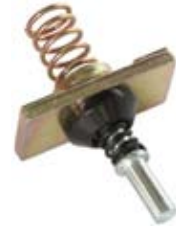
234551 Moving Contact Servicing: 1350-079-01X9, 1350-079-10X9, 1350-084-01X9, 1350-084-10X9, 1350-084-11X9, 1350-084-20X9, 1350-097-00X9, 1350-101-00X9 Th. 5.00, Shaft measurement 31.85 Plate 42.00 x 20.00 x 5.40 mm.
