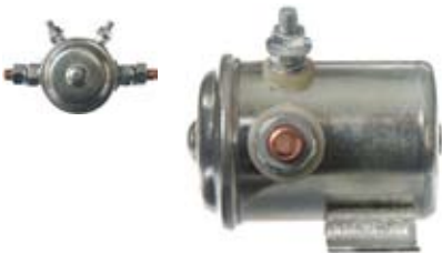
235442 Solenoid Replacing: 1114218, 1114208 12 V., 150 Amp., Intermittent load 300 Amp., Seconds 5 Silver contact. Insulated return.
