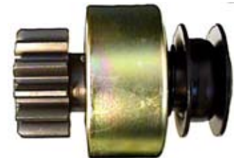
133393 Drive Replacing: 1-23500-0250, 0-23500-0251, 0-23500-0250 Servicing: 0-23000-1160, 0-23000-1231, 0-23000-1270, 0-23000-1601, 0-23000-1660 O.D. 46.54, I.D. 15.00, L. 90.40, Teeth 13, Splines 12, Rotation CR
