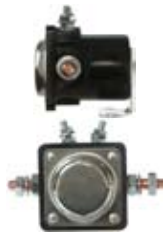
130493 Solenoid Replacing: 3225629, 2098360 12 V., Intermittent load 150 Amp., Coil bolt 5/16" UNF Insulated return. Flat Bracket.
