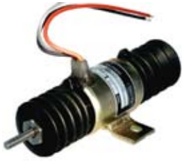
090199 Shut Down Solenoid 12V 12 V., 1.1 Amp., 6.00, Stop solenoid17 Newton178 Newton89 Newton Syncro start / Woodward. Red=Hold, White=Pull, Black=Ground.
