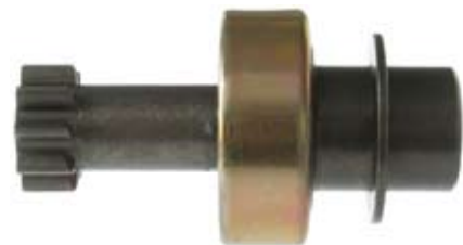
130462 Drive Replacing: 077991 Servicing: D8E103 O.D. 25.25, I.D. 12.00, L. 86.65, Teeth 9, Splines1 12, Rotation ACR
