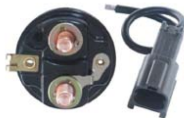
138816 Solenoid Cap Servicing: 2114-87601 O.D. 49.00, Terminals 3
