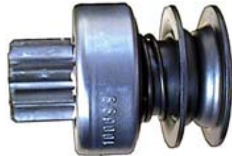
130432 Drive Replacing: 096118, 093297, 092079, 078862, 076651 Servicing: 532005A, 532007A, 532020A, 532020B, 532026A, 533000A, 533002A, 533003A, 533004A, 534003A, 534003B, 534003C, 534004A O.D. 25.25, I.D. 12.00, L. 68.05, Teeth 9, Splines1 9, Rotation CR
