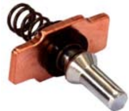
133275 Moving Contact Servicing: M1T70781, M1T70982, M1T71382, M1T72483ZC, M3T30581, M3T30581J, M3T32381, M3T32589, M3T32985, M3T32986, M3T32988 L. 30.05, Th. 2.60, W. 16.00/11.00, Shaft measurement 26.00
