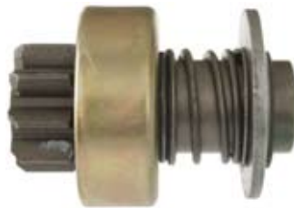
130731 Drive Replacing: 17061-12 Servicing: MTA12-30 O.D. 29.20, I.D. 11.55, L. 61.90, Teeth 9, Splines 12, Rotation ACR
