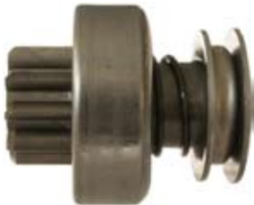
132514 Drive Replacing: 0-23500-0353, 0-23500-0350 Servicing: 0-23000-0031, 0-23000-0032, 0-23000-0040, 0-23000-0060, 0-23000-0060, 0-23000-0100, 0-23000-0240, 0-23000-0330 O.D. 35.30, I.D. 13.00, L. 71.20, Teeth 9, Splines 12, Rotation CR
