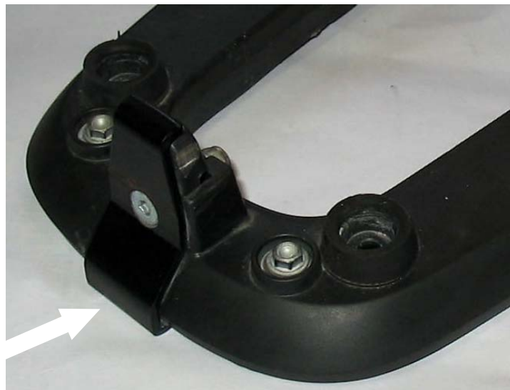
PIC. 2 - Rear Top Case with stiffening brace
