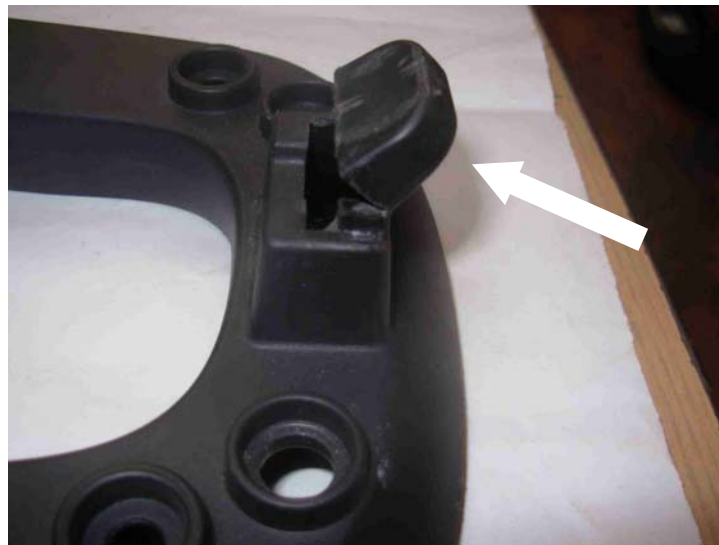
PIC. 1 – Rear Top Case mounting plate with broken tab
