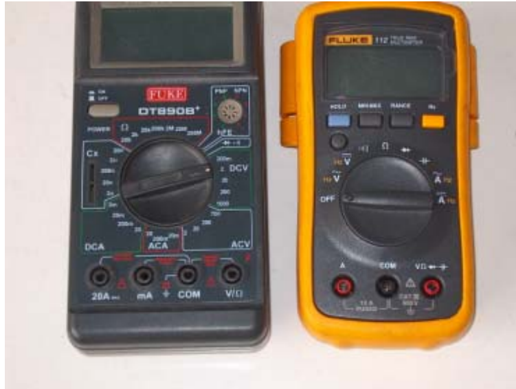
Fig.3 digital multimeter torque on the left side with manual selection and with automatic scale selection on the right side
