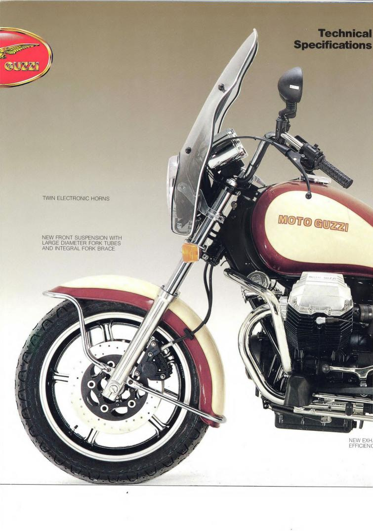
Engine 90° V - twin w/"Nigusil" cylinder lining Displacement 948.8 cc
