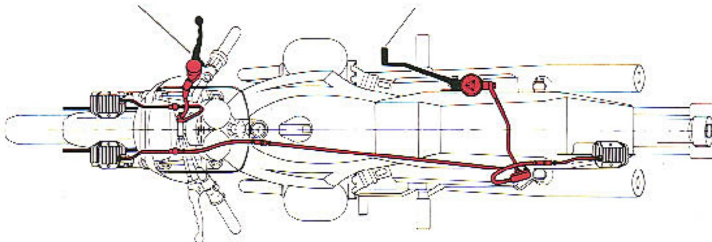
With integral braking system you have the maximum security and stability on the curves and in the wet. The braking movement on the rear wheel controlled by the foot pedal and integrated with a simultaneous braking movement on the front wheel with the distribution
