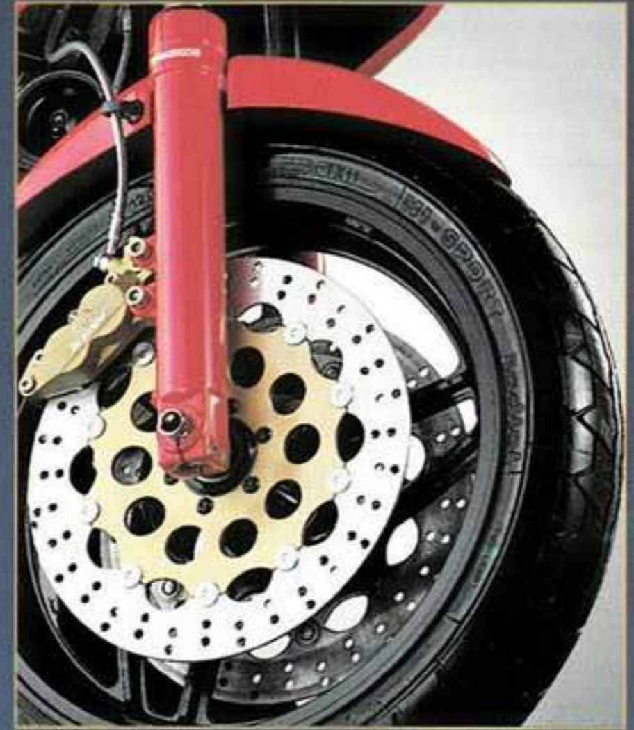
320 mm front disc brakes with four pistons calipers
