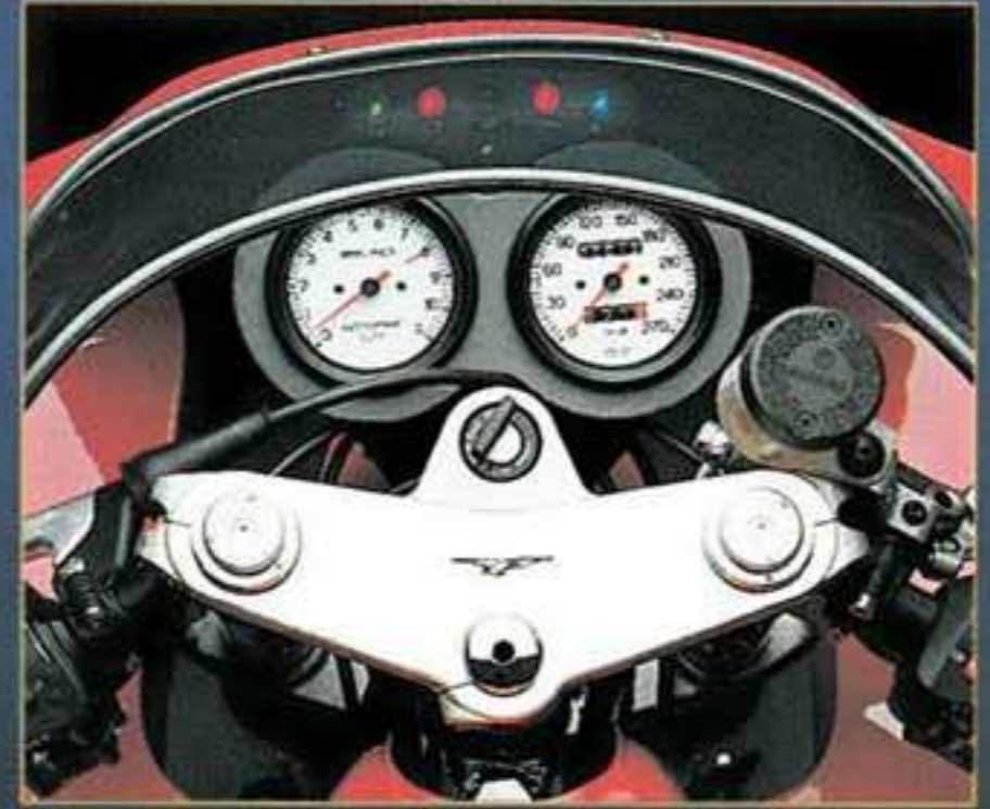
The instruments panel includes: speedometer, rev-counter and warning lights for the main engine operations
