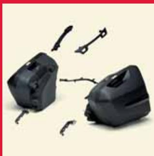
The capacity for long range touring with a passenger is intrinsic to the concept of the Brevia V 1100. Its exclusive luggage system integrates perfectly with the bike, thanks to mounting racks designed to look great even when the panniers are removed. The 29 litre panniers are made with great attention to detail, and come complete with fabric liners to hold all the clothes and personal effects you need to bring that extra comfort to motorcycle touring.
