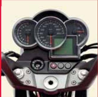
The instruments combine a classic round shape with innovative, advanced functionality. The LCD uses active matrix technology to ensure exceptional clarity under all lighting conditions. While riding, you can interface with the on-board computer without having to take your hands off the handlebars, thanks to controls located at the hand-grips. In addition to all conventional information, the system also reads out maximum and average speed, instantaneous and average fuel consumption.
