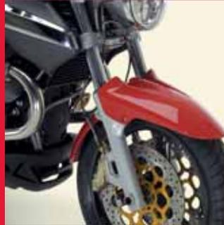
The fork has massive 45 mm stanchions for absolute stability on the straight, precise trajectories into and out of bends, and an extremely responsive ride. Adjustable preload means that you can set up the suspension to suit your own riding style and the road conditions. The front mud-guard integrates with the fork sleeves to improve appearance, creating pleasingly continuous lines and enhancing the dynamics of the design.
