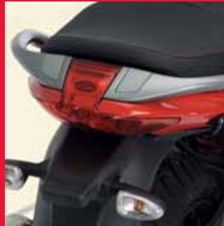
Integrated in the streamlined design of the tail, nestling between the seat and the passenger grab handles, the tail light cluster draws its inspiration from the finest Italian sports car traditions. High intensity LEDs are arranged in circular clusters to ensure maximum visibility from the rear particularly at night, and to give the Breva V 1100 a touch of high-tech style.
