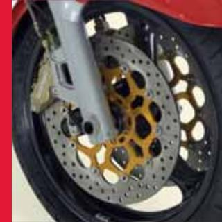
The Breva V 1100's versatility and the great way it adapts to all types of road is achieved in part by two powerful, floating, 320 mm, front discs. The caliper used with this technically advanced unit is equipped with four opposed pistons to tackle late sports braking, emergency stops in traffic, and anything that country roads can throw at you, in total safety. Stopping power at the rear is provided by a 282 mm disc with a floating caliper and two parallel pistons.
