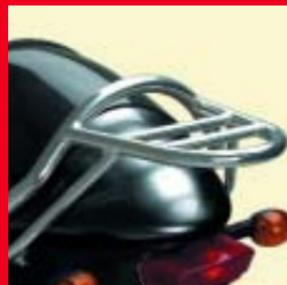
Its design integrates perfectly with the lines of the V11 Sport Ballabio and V11 Café Sport, thanks to the elegant lines and natural anodised aluminium structure. The useful luggage rack is very light and when not in use can be easily removed.
