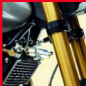
The V11 Café Sport is fitted as standard with an Öhlins fork with solid 43 mm inners and distinctive gilding. Thanks to its particular characteristics, the bike enters bends with precision and follows an ideal trajectory on the straight. The damper on the sensitive and responsive steering also bears the Öhlins signature.
