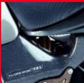
The cantilever swinging fork swingarm fitted as standard on the V11 Café Sport acts on an Öhlins shock absorber, adjustable in compression, rebound and preload. These settings enable the motorcycle to be adapted rapidly to all itineraries and all load conditions, guaranteeing a consistently optimum setup.
