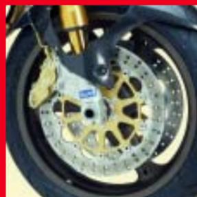
Extreme braking performance and powerful progressive stopping, thanks to the powerful double 320 mm diameter front disc brake, operated by a Brembo caliper with four opposed pistons. A system which adapts perfectly to different riding styles, always offering maximum safety.
