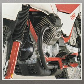
TWIN CYLINDER ENGINE WELL EXPOSED FOR BETTER AIR COOLING
