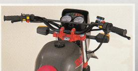
INSTRUMENTAL PANEL CONSISTS OF REV-COUNTER, A SPEEDOMETER WITH TRIPMETER AND WARNING LIGHTS
