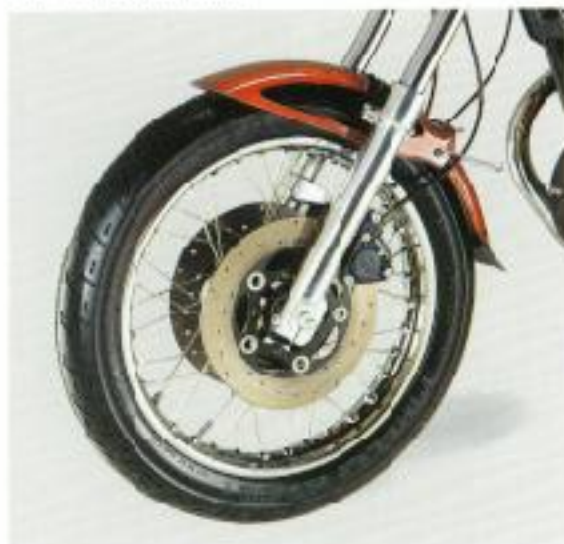
FRONT DOUBLE FLOATING DISC BRAKES FOR 750 NEVADA ONLY
