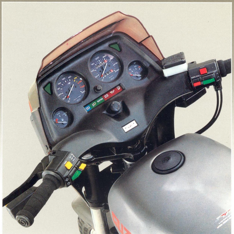
INSTRUMENTS ENCLOSED IN COCKPIT FAIRING INCLUDE SPEEDOMETER WITH TRIP METER, REV-COUNTER, VOLTMETER, FUEL LEVEL INDICATOR AND WARNING LIGHT PANEL
