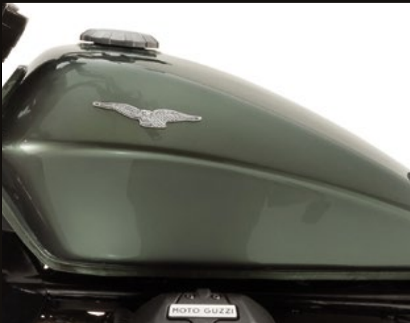
STEEL TANK WITH EAGLE IN RELIEF
