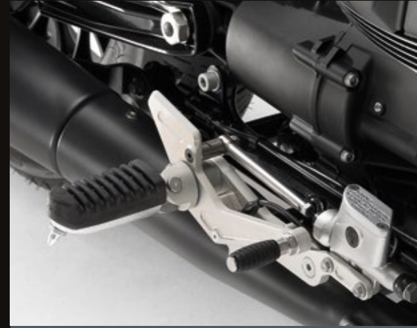
ALUMINIUM FOOTRESTS AND SUPPORTS
